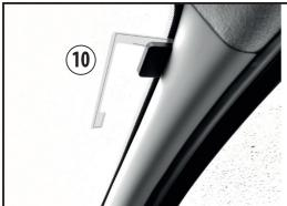
Install the DAB+ antenna on the right-hand side of the windscreen, ensuring the bronze section touches the vehicle's frame (this is necessary to power the antenna).
