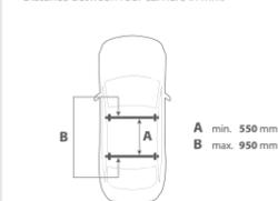
Maximum width roof bars mm:
