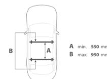
Maximum width roof bars mm:
