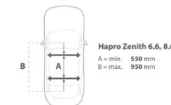
Maximum width roof bars mm:
